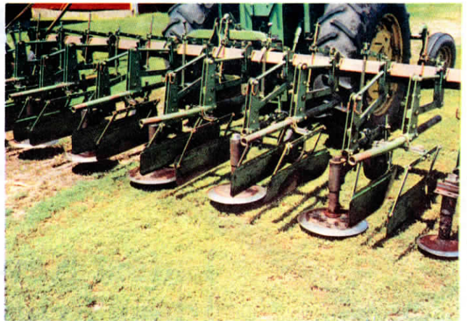
Flitter removed the shovels from each cultivator gang, replacing them with one 18-in. disc blade per row.
