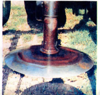
Blade mounts on "spindle", made out of steel tubing, that turns inside a larger piece of pipe which acts as a greasable "bearing".
