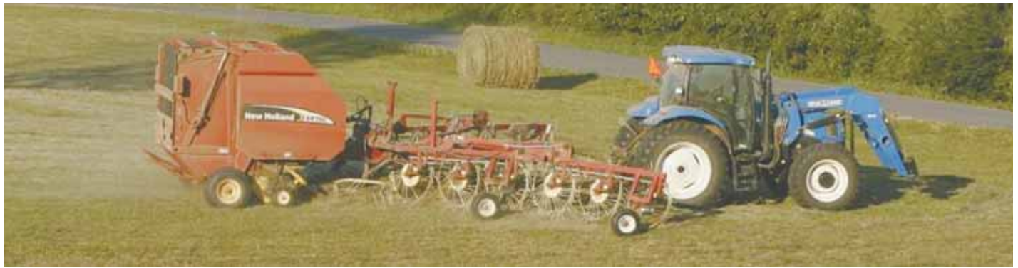
You can rake and bale hay in one pass with the Rake-N-Roll, built by Bruce Peden and his brother Don. The 12-wheeled, V-shaped rake fits between a tractor and baler.
