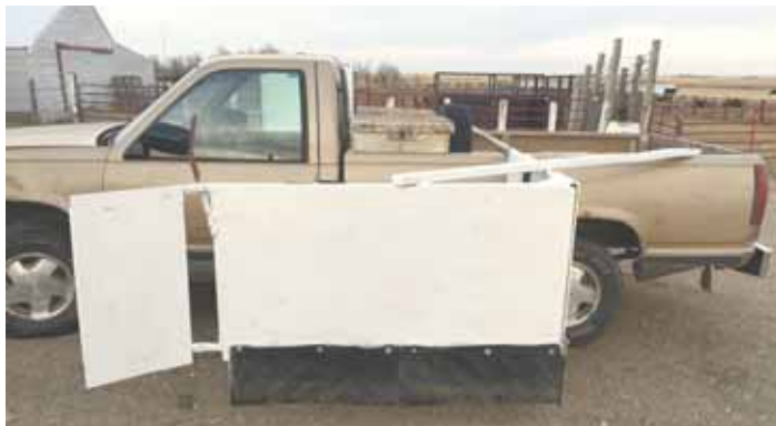
Pickup-mounted calf catcher lets Don Karst catch spray calves without concern for mad mamas.
