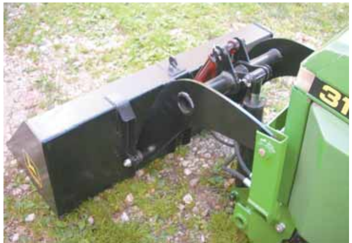
Loader operates off tractor’s standard onboard hydraulic system.
