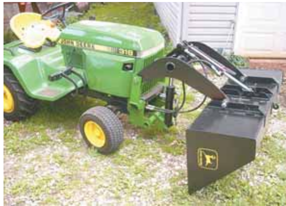
Loader’s boomerang-shaped lift arms are raised or lowered by a single hydraulic cylinder. Another cylinder is used to tilt bucket.
