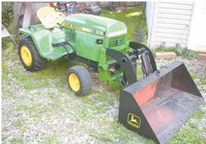
“It worked great for removing snow last winter,” says Steve Nichols about the mini loader he built for his Deere 318 garden tractor.
