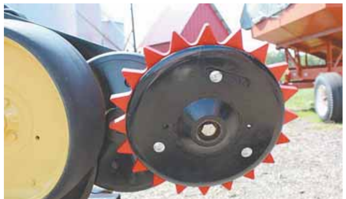
Gerald Milo and his son built unique cog-type closing wheels for their no-till drill that improves seed stands.
