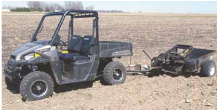
Hydraulic-powered Marshall Picker tosses rocks into a cargo box with a 12-volt hydraulic-powered reel.
