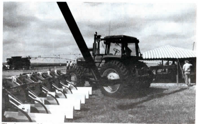
Thanks to new hinge, toolbar folds flat to reduce overall transport width.
