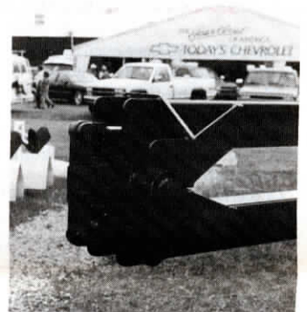
Each hinge is fitted with two cylinders which provide the 180° folding action.
