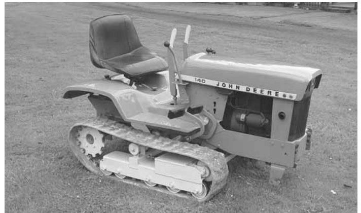
Bob Gauntt mounted the tracks off an old Chinese-built manlift on a Deere 140 riding mower to come up with this tracked tractor.
