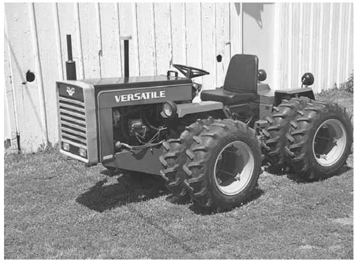
Tractor is complete with fully functioning hydraulics and 3-pt. hitch. The grill was made from 3 lawn tractor grills, cut up and reassembled to size.
