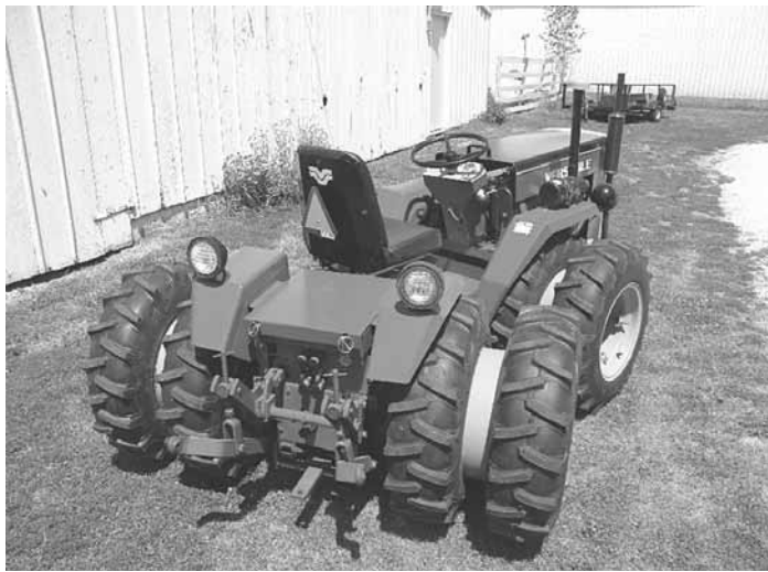
Instead of the 200+ hp Cummins engine common to full-size Versatile tractors, Ted Huber's articulated Versatile 824 is powered by a 24 hp Yanmar.
