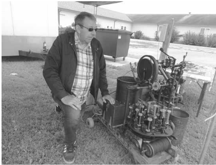
"I often demonstrate my antique braiding machines at local antique tractor shows, where they're a big hit," says Al Kamminga. The 2 machines ride on wheels and at shows stand side by side, belt-driven by the same electric motor.
