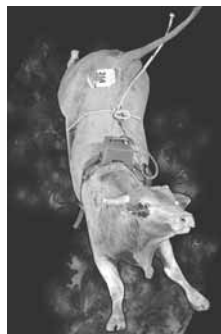
Dummy is placed on bull in chute and turned on or off remotely.
