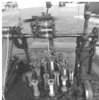
Each braiding machine uses a series of 16 "bobbins" that work by means of a circular weaving process.
