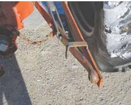
L-shaped steel brackets keep stabilizer bars in place on tractor's 3-pt. lower lift arms, even when the 3-pt. isn't hooked up to an implement.
