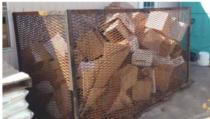
Skid loader-mounted burn cage measures 9 ft. long by 5 ft. 2 in. high by 5 ft. deep. "It can be easily moved to a safe area for burning and is big enough to save a lot of time and labor," says Marion Schrock.
