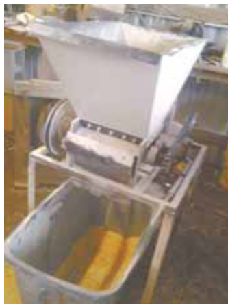
Homemade roller mill sets on angle iron legs with room to slide a bucket underneath (left). Rollers are 4 1/2-in. outside dia. pipes with grooves cut in them at 1/4-in. spacings.
