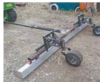
Jacob also built a pull-type magnet that can be used around construction sites, landfills or farm yards.
