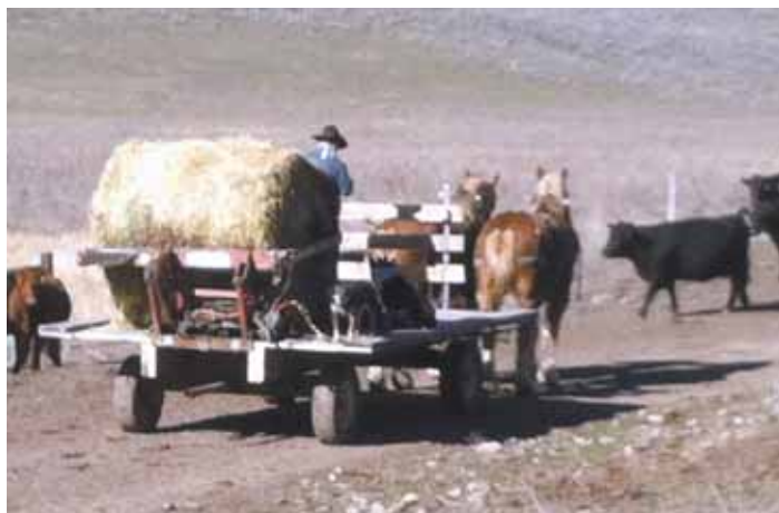
Bart Spear's wagon-mounted DewEze bale handler makes it easy to feed out 2 big bales at a time. He uses a single team of horses to pull it.
