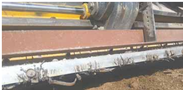
Terry Jacob's road grader has a 12-ft. permanent magnet mounted behind the blade and separate from it.
