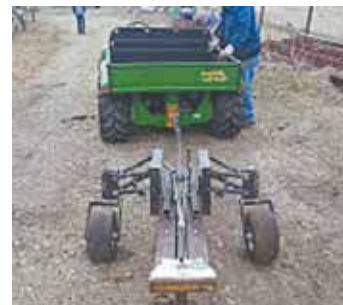
Jacob also built a pull-type magnet that can be used around construction sites, landfills or farm yards.
