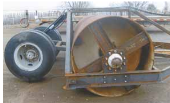
He started with 2 scrapped and gutted drums that came from a self-propelled asphalt roller. They were 7 ft. long and about 4 ft. in dia.
