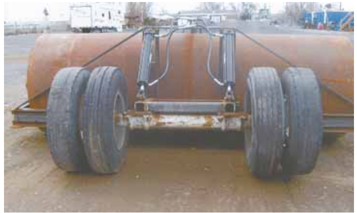
He started with 2 scrapped and gutted drums that came from a self-propelled asphalt roller. They were 7 ft. long and about 4 ft. in dia.
