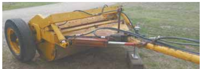
Terry Jacob converted a road packer into a field roller that he pulls behind a levee-terracing plow. It makes flat paths in fields for pivot wheels.
