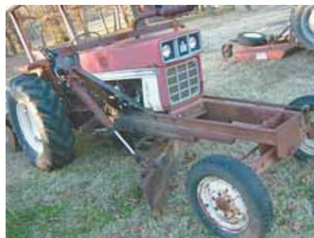
Allen Kimball built this belly-mounted blade for his IH 284 tractor. "It grades driveways smooth without washboarding," he says.
