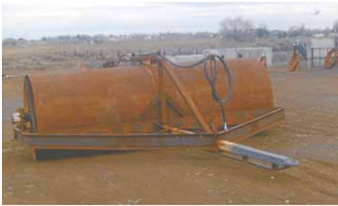
Alan Heilman used scrap metal to build this field roller for his brother-in-law. It's about 15 ft. wide and just over 20 ft. long.
