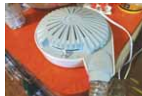
Modified hair dryer forces air through a pair of pvc pipes to dry boots.
