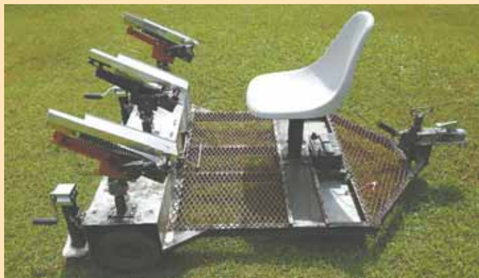
Each thrower can be quickly adjusted to one of 10 different angles, and then locked in place with set screws.
