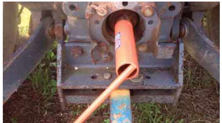
"Easy Turner" makes it easy to line up your tractor pto with an implement. It consists of a short length of pipe with a steel peg welded on inside to grab a spline. A metal rod welded to one end of pipe serves as a handle.
