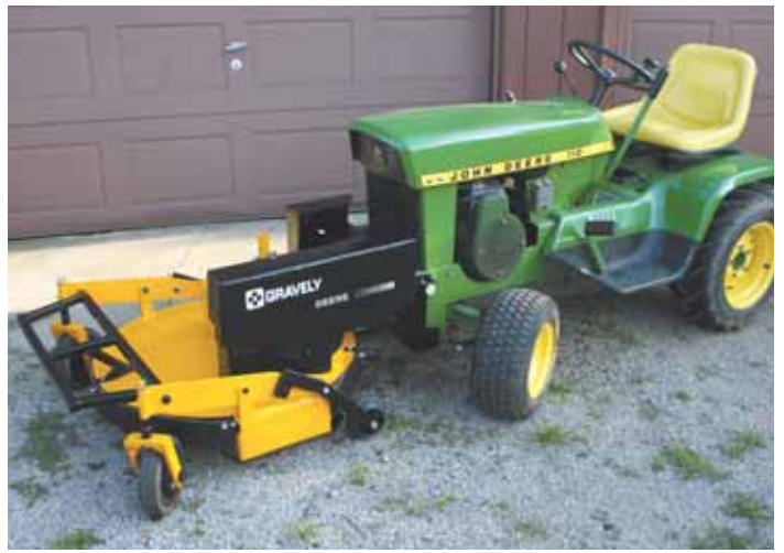
He designed a mounting bracket with a pulley drive that uses the tractor's belly mower drive system.
