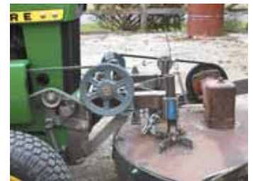
Pulley driveshaft transfers power from tractor's right side to the left to line up with the Gravely deck.
