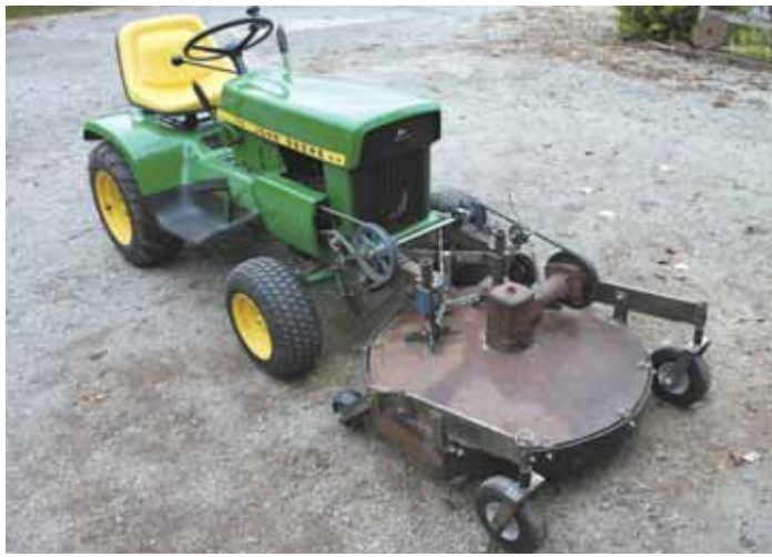
Reid Prinkey mounted the rotary deck off a Gravely walk-behind mower on front of his Deere garden tractor. It chews up small trees and brush and also mows his lawn.
