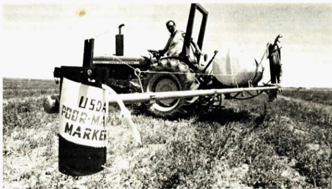
A tug on the rope ejects a blob of easy-to-see shaving cream.
