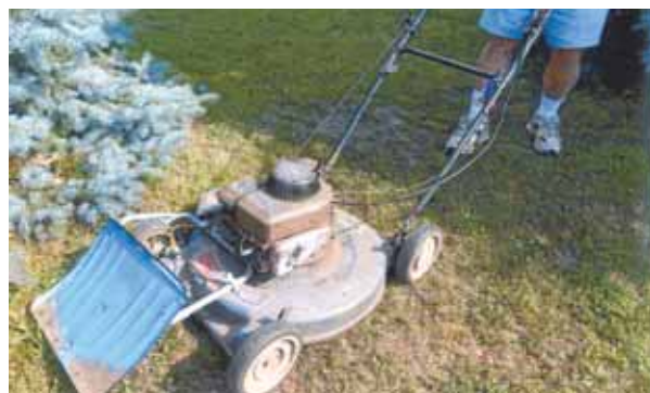
Chuck Hampe uses a snow shovel blade mounted on front of his push mower to lift branches out of the way as he mows.
