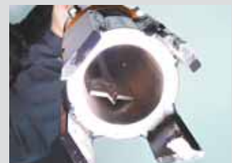
Unit is available with 2 cutting heads for digging 4 and 8-in. dia. holes (left). Dirt is vacuumed up tube and into canister. A thresher blade inside head breaks up any plugs.
