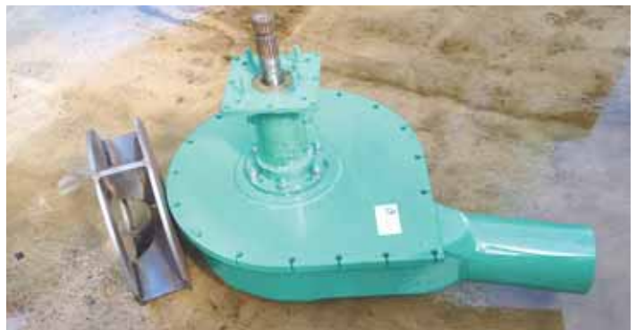
B&M Welding says its replacement pump for big liquid manure tanks pumps faster and lasts longer. Photo shows pump housing with bearing housing and shaft impeller at left.
