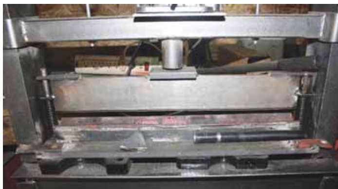
"I've used this brake to make hundreds of bends, and it's still in excellent shape," says Kevin Ranette about the metal brake he built to fit his 20-ton shop press.
