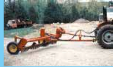
Rock Rake Made From Baler Parts (See page 26)
