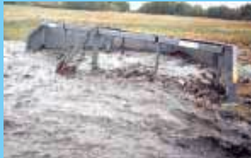
“Drag” Drains Sloughs & Potholes (See page 20)
