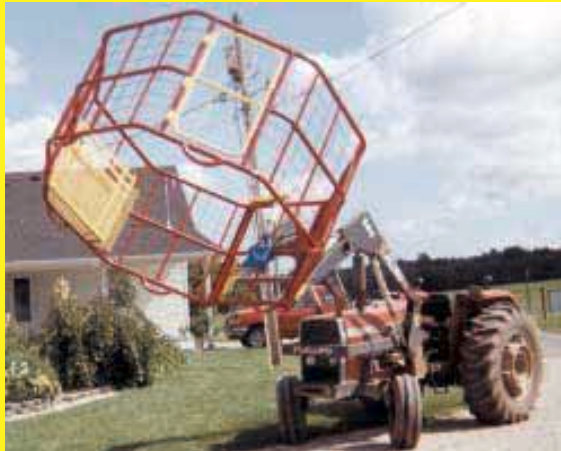
Tractor-Mounted Calf Catcher - After a mother cow nearly stomped him to death, Kentucky cattleman Larry Jeffries came up with this calf catcher to fit his front-end loader. The portable corral is equipped with a weigh scale and calf chute. See page 2.
