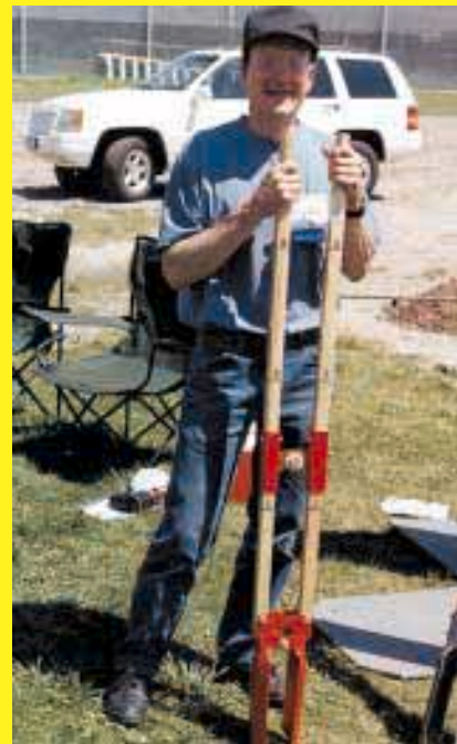
New-Style Posthole Digger - What makes Jeff Vaughter's new posthole digger different is the pivot point a couple feet up from the jaws. The handles never spread out wider than the hole being dug. See p. 3.
