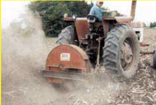
Field Ditcher Made From Silo Blower - Kansas farmer Elwin Harder cut off the bottom of a silo blower to make a 3-pt. mounted low-cost ditcher. He uses it to drain surface water off fields. See page 2.
