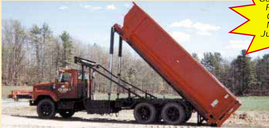
Roll-Off Garbage Containers Haul Forage - New Hampshire farmers Russ Atherton and Tom Morrell have started using big roll-off garbage containers to haul forage in from the field. They park a 50-yard container at the side of a field and dump into it with a side dump wagon. A truck then hauls it back to the farm at highway speeds. See page 2.
