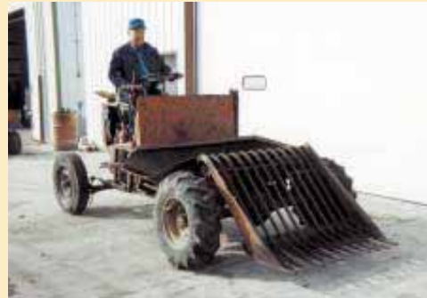
Self-Propelled Rock Picker - Minnesota farmer Wayne Juhl didn't like his commercial rock picker so he built this 3-wheeled, self-propelled rig with a rock picking bucket positioned between the front wheels. It tilts back to dump into a steel hopper which dumps to the side when full. See page 2.
