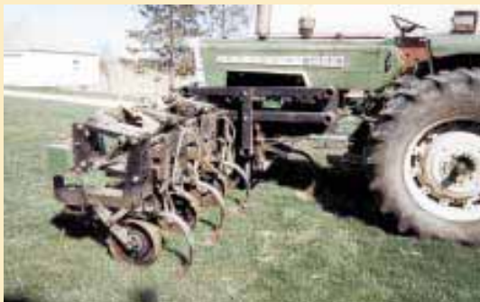
Front-Mount Cultivator - Iowa farmer Jeff Gravel converted a standard rear-mount cultivator to mount on front of his tractor. Cultivator fastens directly to front of tractor without a 3-pt. hitch, which Gravel felt would have put the cultivator out too far in front of tractor. See page 3.
