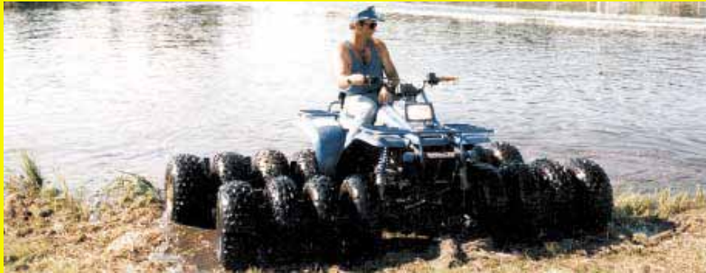
16-Wheel ATV Runs Through Water - Gene Riddlestine didn't like the fact that he had to stop at the edge of the water with his ATV. So he added 12 wheels to the bike, more than enough to float it in water. To help propel the bike, he fitted small paddles to the steel spacers between each set of wheels. See story on page 2.
