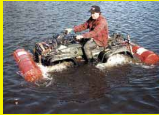
Amphibious ATV Fitted With Floats - Mike Dick welded steel drums together to make big floats for the front and back of his ATV. He wanted to be able to cross rivers and lakes when hunting or trail riding. See story on page 2.
