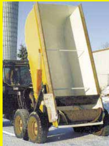
Spreader raises straight up to vertical to completely empty out. Note home-built beater at bottom.
