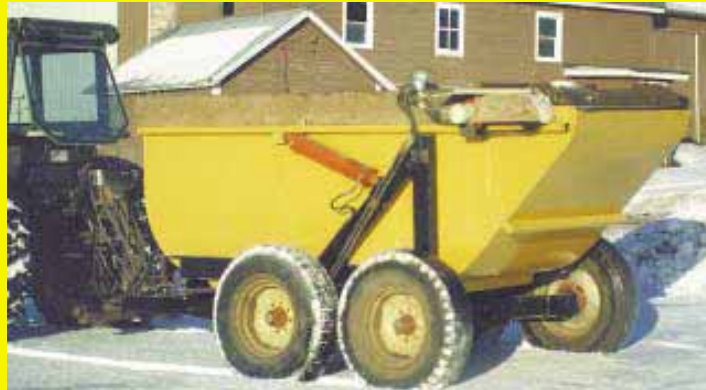
Lloyd Bauer built this 2,000-gal. spreader for only about $2,000. It's lined with a spray-on "slippery" plastic that helps manure slide out freely.
