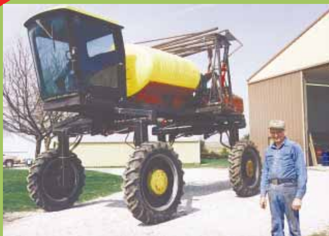
Marshall Litchfield's "variable clearance" sprayer hydraulically raises and lowers from 3 to 6 ft. off the ground, allowing him to use it for all his spraying jobs from early spring to late summer. Axles pivot independently to provide articulated steering.
