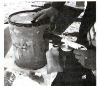
Rubber blasting tip, which reclaims sand, strips clean an area the size of a quarter. Sells for $110. Uses normal sand-blasting sand. Contact: FARM SHOW Followup, Pres-
