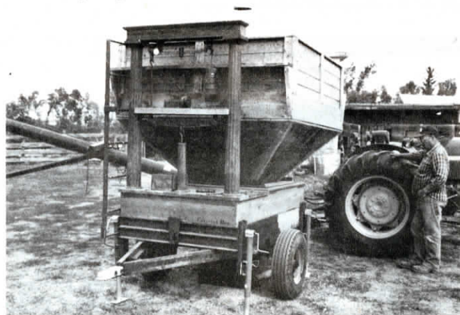
Guth mounted salvaged elevator scale on wheeled chassis to weigh grain, fertilizer.
