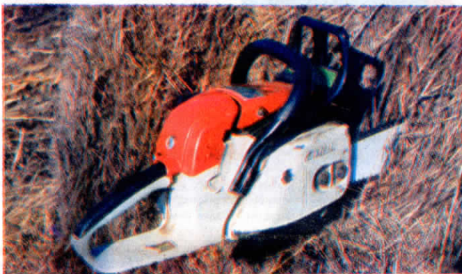
Bale-cutting saw chain lets you cut up round bales into smaller pieces that are easier to handle. Slicing up bales also makes it easier for cattle to tear off hay, reducing waste.
