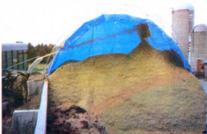
Silo blower loads silage into "shaper". Photo shows model designed to mount on walls of existing bunker silo.
