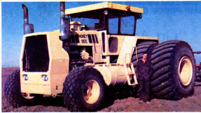
Home-built tractor's Cummins diesel engine, rated at 700 hp, was scaled down to 425 hp.
