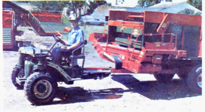
Trail Blazer automatically couples to implements.
