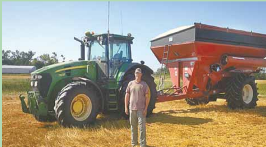
Manitoba farmer Matt Reimer uses an electronically steered tractor to pull his grain cart, controlling the tractor on-the-go from a laptop computer inside his combine. He assembled the system himself.
