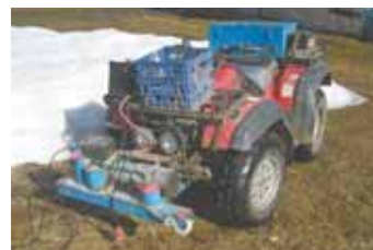
He also installed a bigger bumper to support a bigger winch, which is powered by a 12-volt automotive battery mounted on back.
