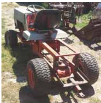
He lengthened the frame by 2 ft. and also welded a cross piece on back to support the dump bed.
