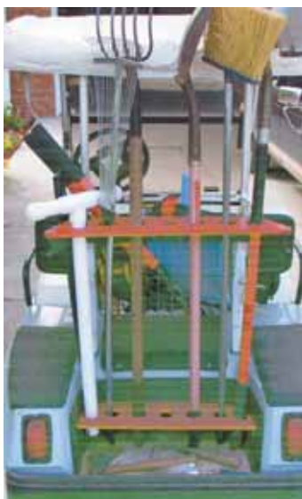
Robert Lord modified his golf cart to carry up to 7 different garden tools.
