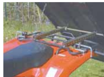
Box mounts on a pair of rails bolted to ATV's rear cargo rack.
