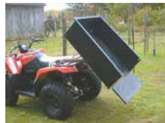
Rich Ferfecki unbolted the box from a small wagon and mounted it on back of his ATV, converting it to a handy dumping cargo box.
