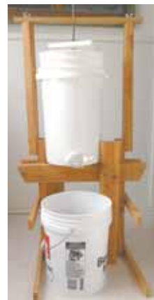
Using a plastic pail and an electric drill to power a spinner, James Noble is able to extract honey without damaging the comb.
