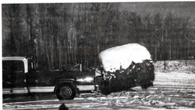
Sherstan lifts each bale off the ground with the rear bale forks, which are powered by an 8,000-lb., 12-volt winch. A 3-in. stroke cylinder, mounted in-line between the winch and the bale forks, acts as a load cell (below left). A single 12-ft. hydraulic line runs from the cylinder to a standard pressure gauge in the cab where Sherstan reads the bale's weight (below right).
