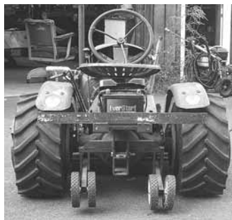
Tom Demers turned an old Panzer garden tractor into a pulling tractor, adding a pair of 10-in. high wheelie bar wheels on back.
