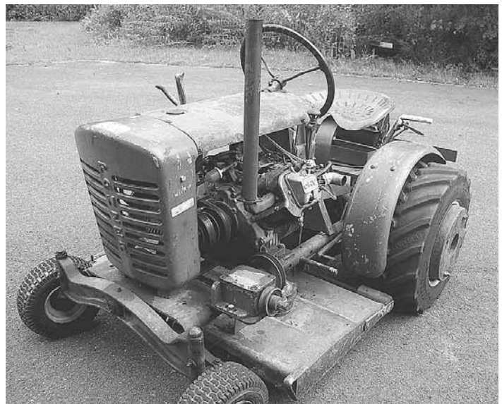
He replaced the Panzer’s engine with a 9 hp Kawasaki engine but kept the mower deck, which weighs 150 lbs., for added traction.
