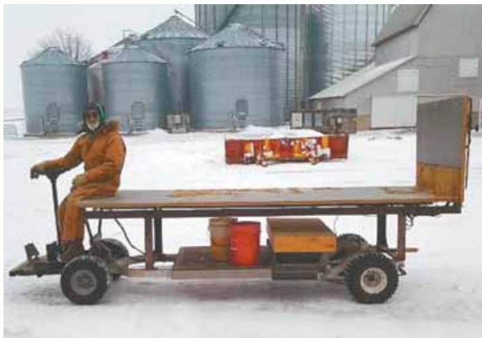
Paul Butler converted a Club Car 6-passenger, electric-drive golf cart into this “big bale cart” that handles big square bales weighing up to 800 lbs.
