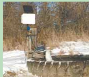
Kit attaches to a standard water hydrant. Schirado can fill the tank with a text from his cell phone.
