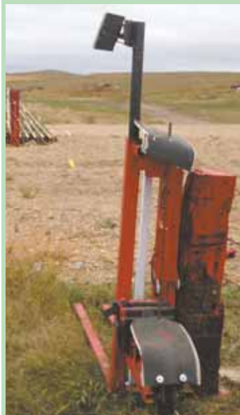
Remote-controlled gate uses a solar-powered linear actuator to hold, release and reattach the gate post, which is hinged at ground level.
