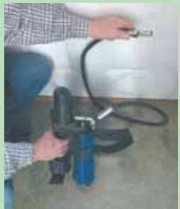
A trigger at the end of the hose makes it easy to apply grease with one hand.
