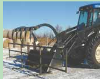
Schirado uses loader-mounted bale forks to lift his home-built gate out of the way, then drives through and sets it back down. The 4-ft. long feet give gate stand-alone stability.
