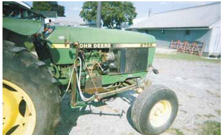
Merle Martin uses the side-step mounted boom on his tractor to spray road ditches, fence lines and field edges.
