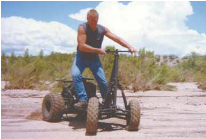
David Zuhlsdorf made this stand-up, off-road 4-wheeler by crossing a scooter with an ATV.
