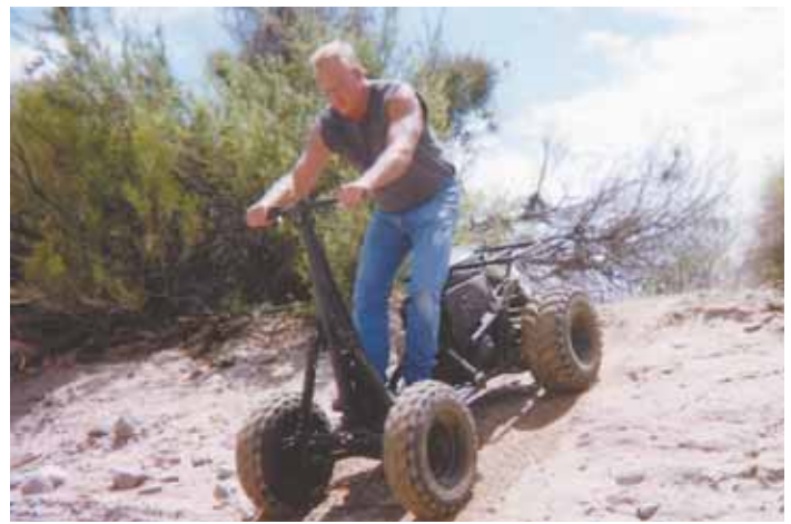
The 4-wheeler's front and rear ends have independent frames connected at a pivot point. "The front end can twist one way and the back another," says Zuhlsdorf.
