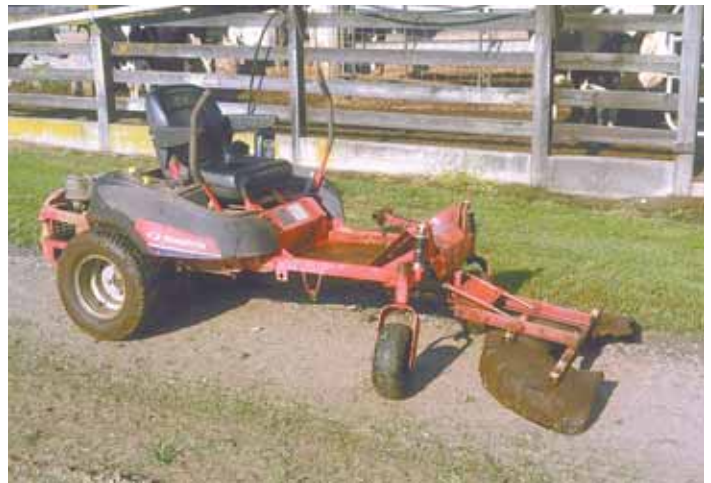
Dave Wampler turned an old zero-turn riding mower into a handy barn scraper. "It has enough speed and maneuverability to make barn cleanup easy," he says.
