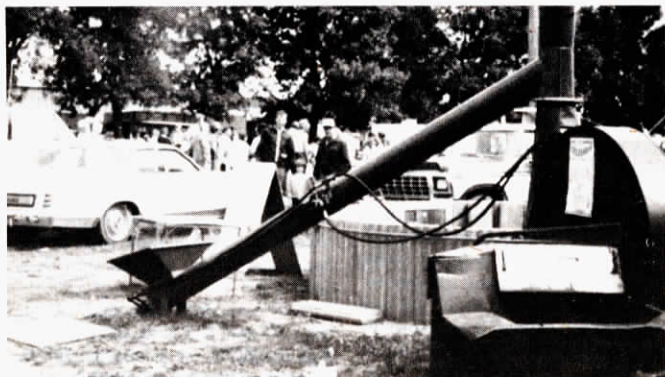
The Auger Blower attachment fits between the permanent silo pipe and the blower neck. It intercepts pressure from the blower fan to move grain without cracking it.
