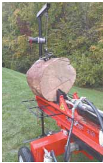
“Drag and lift” system drags logs weighing up to 250 lbs. to the splitter and lifts them onto the splitter beam. A screw ring screws into the log and is attached to a cable hook. A 12-volt electric winch cranks up the cable.
