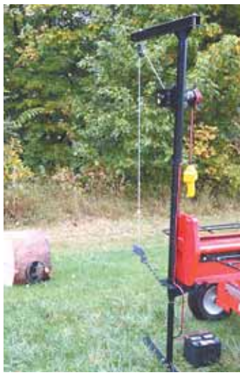
“Drag and lift” system drags logs weighing up to 250 lbs. to the splitter and lifts them onto the splitter beam. A screw ring screws into the log and is attached to a cable hook. A 12-volt electric winch cranks up the cable.
