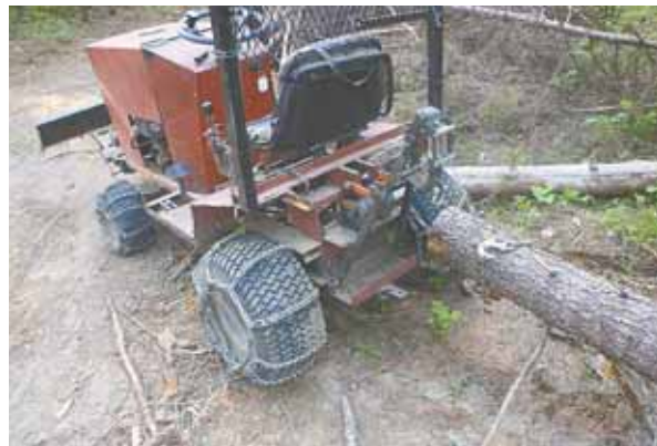
Kevin Ranette’s home-built “logging tractor” has a 40-in. wide, 16-in. high blade on front that’s raised and lowered by an electric winch.
