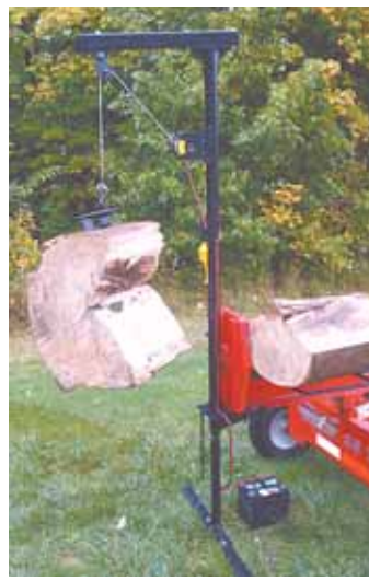
“Drag and lift” system drags logs weighing up to 250 lbs. to the splitter and lifts them onto the splitter beam. A screw ring screws into the log and is attached to a cable hook. A 12-volt electric winch cranks up the cable.
