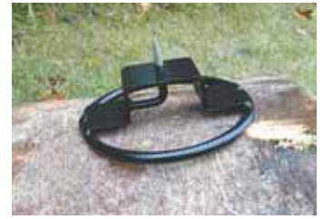
“Drag and lift” system drags logs weighing up to 250 lbs. to the splitter and lifts them onto the splitter beam. A screw ring screws into the log and is attached to a cable hook. A 12-volt electric winch cranks up the cable.
