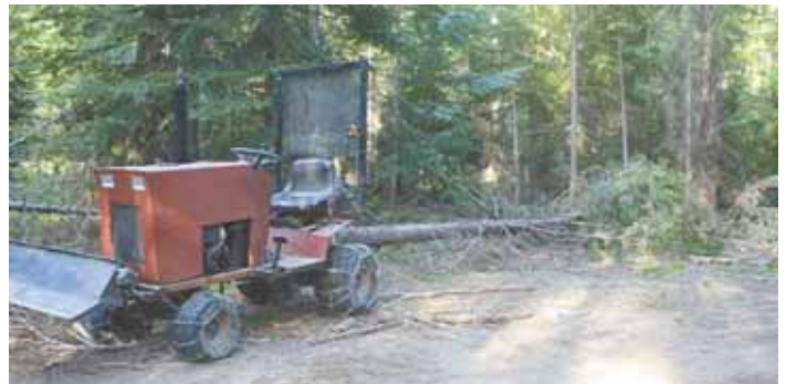
Kevin Ranette’s home-built “logging tractor” has a 40-in. wide, 16-in. high blade on front that’s raised and lowered by an electric winch.
