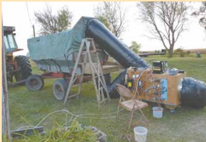
Joe and Dave Loebach dehumidify grain rather than heating it. To test the idea, they installed a dryer floor in the bottom of a flare box wagon with a tarp over the top to seal it. A blower cycles oxygen-deprived air through the system.
