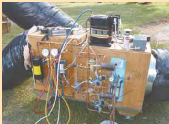
Joe and Dave Loebach dehumidify grain rather than heating it. To test the idea, they installed a dryer floor in the bottom of a flare box wagon with a tarp over the top to seal it. A blower cycles oxygen-deprived air through the system.
