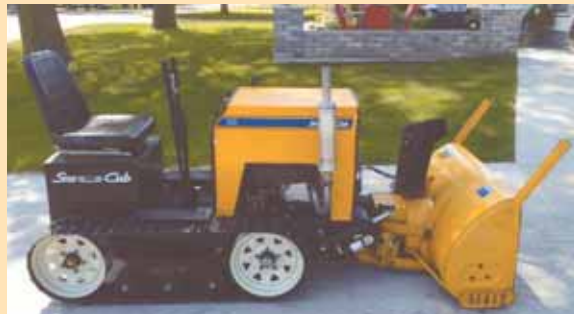
"Sno Cub" rides on a pair of 7 1/2-in. wide tracks made by cutting an old Polaris snowmobile track lengthwise in half.
