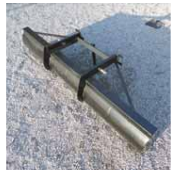
Mark Yax's home-built snow blade mounts on the lift arms on back of his Ford 8N tractor, allowing him to pull snow away from buildings.
