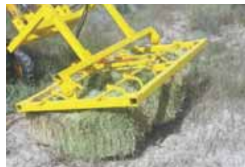
Chris Kornkven saved money by building this self-leveling square bale grapple fork for his Case skid loader. It's designed with 12 bale hooks and can pick up 4 or 5 bales at a time.
