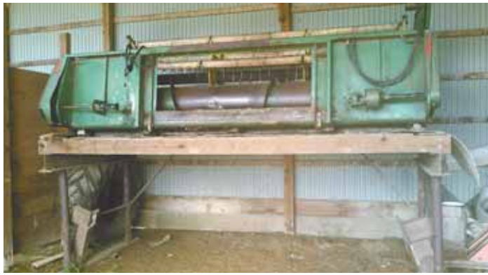
The 16-ft. long deck sits about 5 ft. off the shed's floor. The Wamplers store their grainhead on top of the rack and their 4-row cornhead underneath it.
