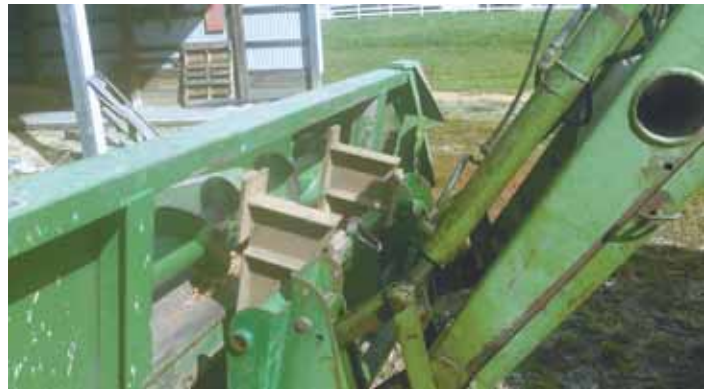
Homemade grab bars on their loader allow Dave and Keith Wampler to snatch up combine headers and quickly stack them on or under the header deck in their shed.
