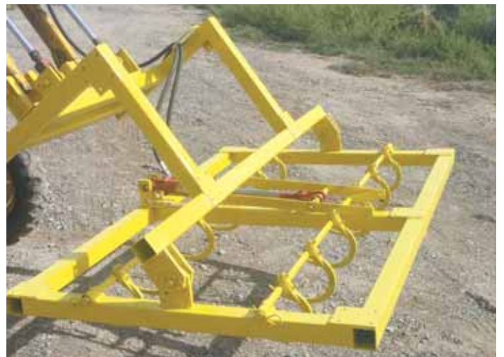
Straw chopper can hold several small square bales or sections of big square bales. As tray tips up and locks into position, bales feed down by gravity into a rotor.
