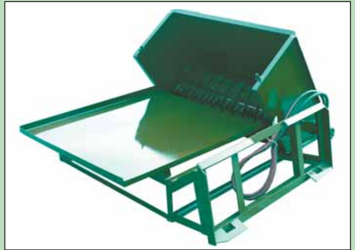
Straw chopper can hold several small square bales or sections of big square bales. As tray tips up and locks into position, bales feed down by gravity into a rotor.
