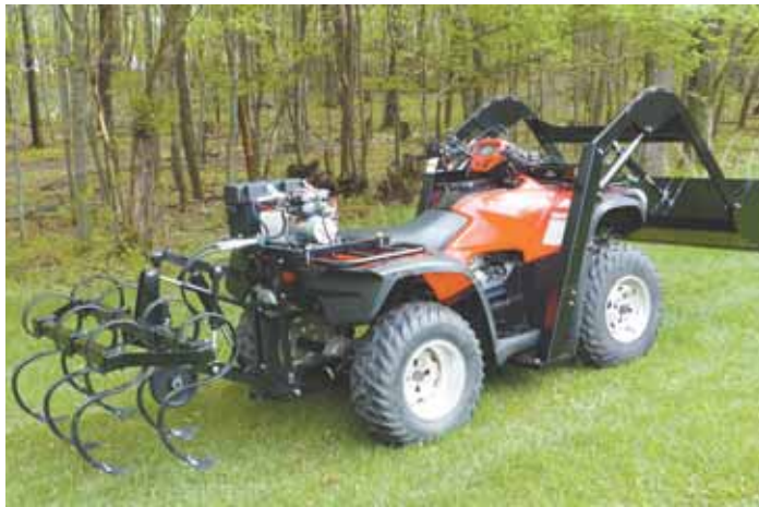
Jim Ruen likes the loader and 3-pt. mounted cultivator mounted on his Honda Foreman 4-wheeler. Replacement parts are now available from Wild Hare Mfg.
