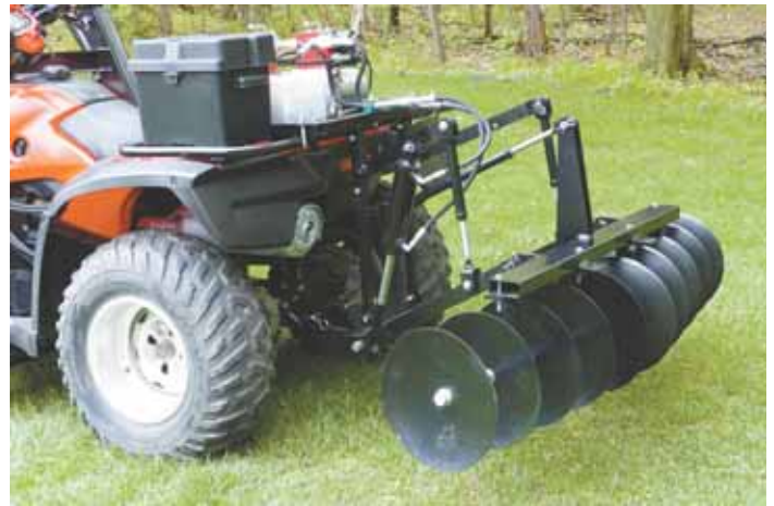
Some of the Wild Hare accessories available include this rear 3-pt. hitch and 57-in. disk harrow, as well as a battery box.
