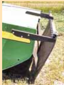
Rock Block curtain mounts ahead of rotary mower/conditioners to keep rocks from being thrown forward toward tractor. Sections fold forward for easy access to machine.
