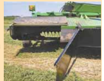
Rock Block curtain mounts ahead of rotary mower/conditioners to keep rocks from being thrown forward toward tractor. Sections fold forward for easy access to machine.
