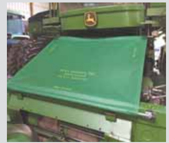
Measuring 4-ft. square, the vinyl Debris Deflector keeps debris from collecting on top of combine's feederhouse.
