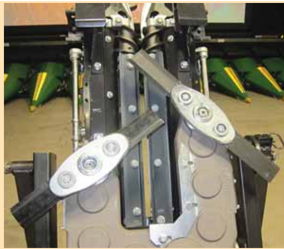
New Twin Chopper option features 2 counter rotating blades, one located slightly ahead of the other to provide maximum coverage and stalk breakdown.
