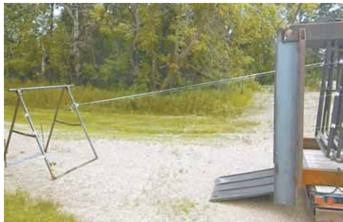
A-frame fence stand allows an operator to anchor wires to a post or tree and then drive along dispensing frames and wire as they go.
