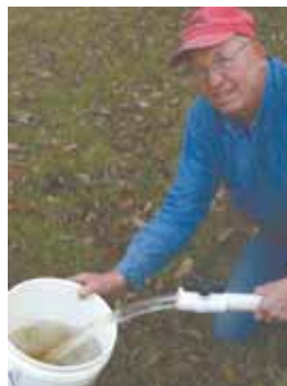
Built in 10-ft. sections, the siphon connects easily for setup and breaks down quickly when done. Photo above shows siphon components.
