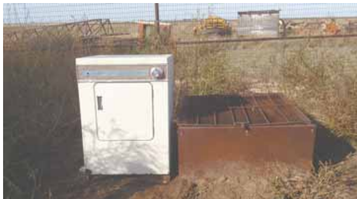
Donald Dean Sarchet burns his trash in a 30-ft. deep hole in the ground with help from a discarded clothes dryer that blows air deep into the trash for a complete burn. A stovepipe connected to the dryer vent runs down into the hole.
