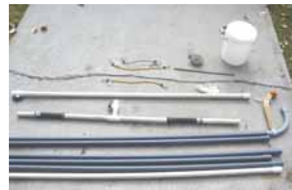
Built in 10-ft. sections, the siphon connects easily for setup and breaks down quickly when done. Photo above shows siphon components.
