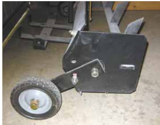
Doug Creswell wanted to transport his tow-behind box scraper from his barn to a work site without scraping along the way, so he added a pair of 6-in. rubber wheels on back.
