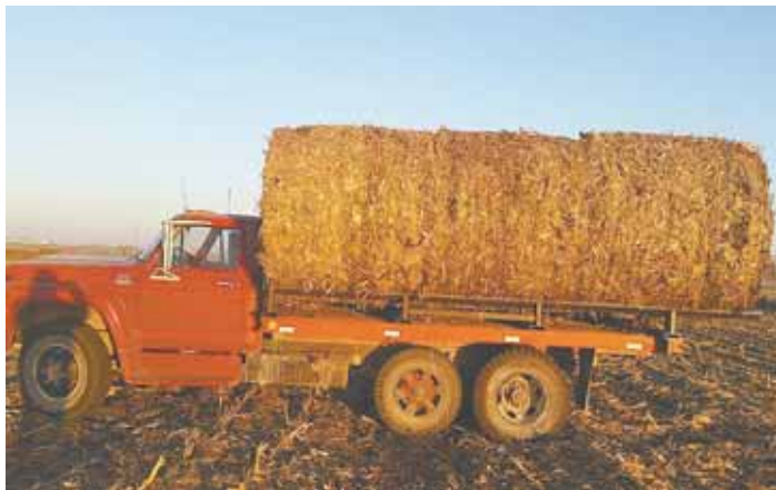
Bolt-on, bale-holding frame replaces the grain box on Matt Abbas's old Ford F-600 2-ton truck. It can haul 6 round cornstalk bales at a time.
