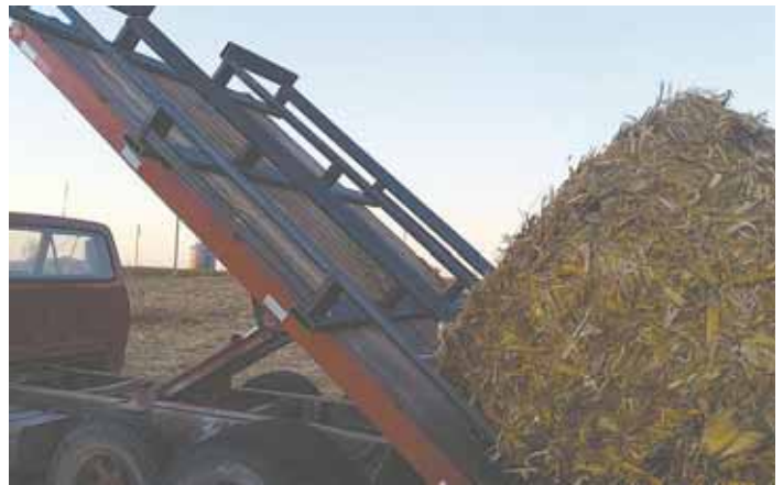
Abbas uses the truck's hoist to slide bales off the back end of frame.
