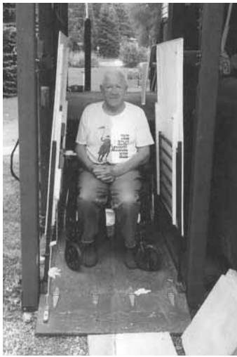
Goertzen's wheelchair lift uses a 12-volt ATV winch with steel cable to do the lifting. Operator pulls an overcentered lever to lock hinged ramp in upright position.
