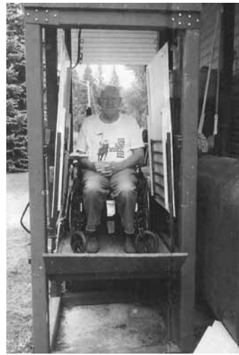
Goertzen's wheelchair lift uses a 12-volt ATV winch with steel cable to do the lifting. Operator pulls an overcentered lever to lock hinged ramp in upright position.
