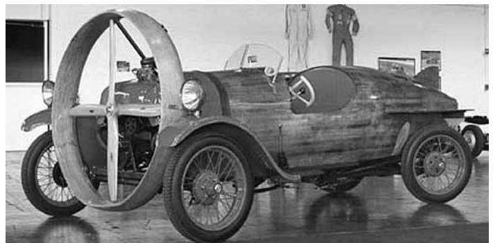
At the front of the torpedo-shaped body is a 4-cyl. air-cooled Citroen GS engine with a 3-ft. dia. double shaft propeller coupled directly to the crankshaft.
