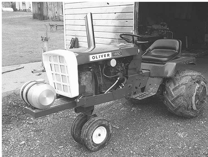
Matt Frank turned a Simplicity garden tractor into this diesel-powered, mini Oliver 1650 with a narrow front end. He says it holds its own at tractor pulls.
