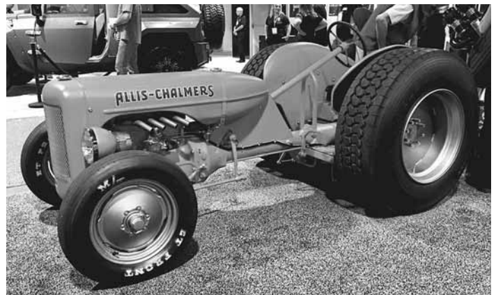
Eric Del Ponte built this Allis Chalmers “dragster” by modifying a 1939 Allis Chalmers B, lowering the axles and adding big rear wheels and tires off a semi truck.
