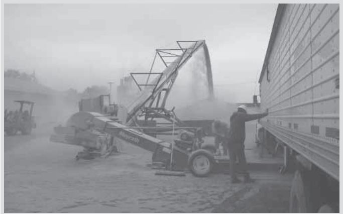
Scott Cerveny likes the Hutchinson 70-ft. squeeze belt conveyor he uses at the Aurora Co-Op in Aurora, Neb. It can easily move 8,000 to 12,000 bu. of grain per hour.
