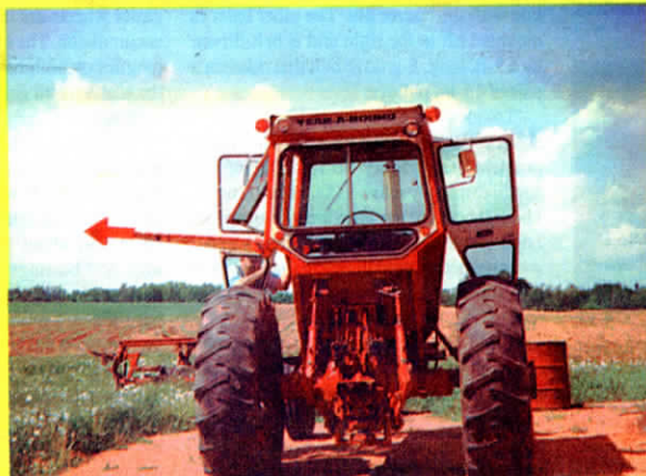
When not in use, turn signal arrow points straight up (top). To make a left turn, Damrow drops arrow down, which completes electric circuit, activating red flasher light on tip of arrow.
