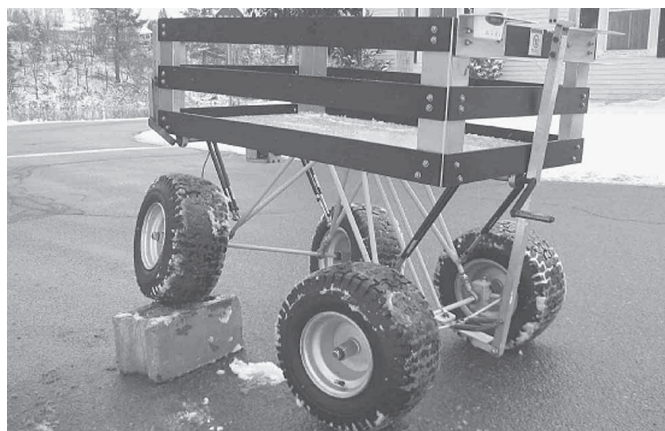
Wagon rolls on large diameter pneumatic tires that allow it to smoothly walk over large objects. Front-mounted manual crank lowers rear tailgate, which children climb up.
